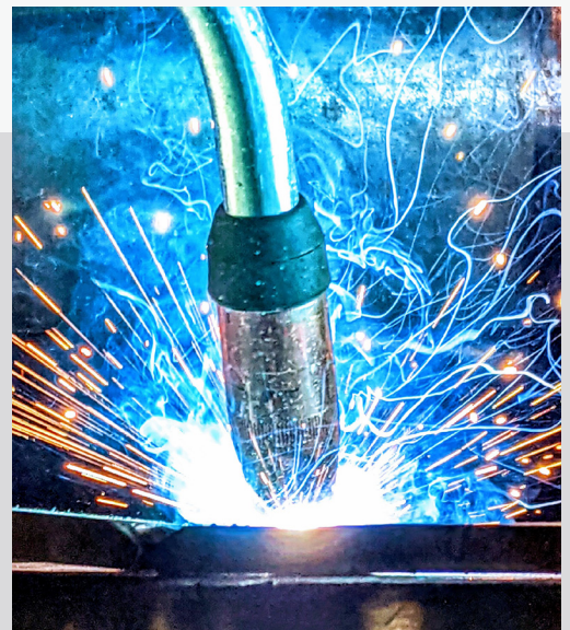
Spray pulse MIG welding in action.
