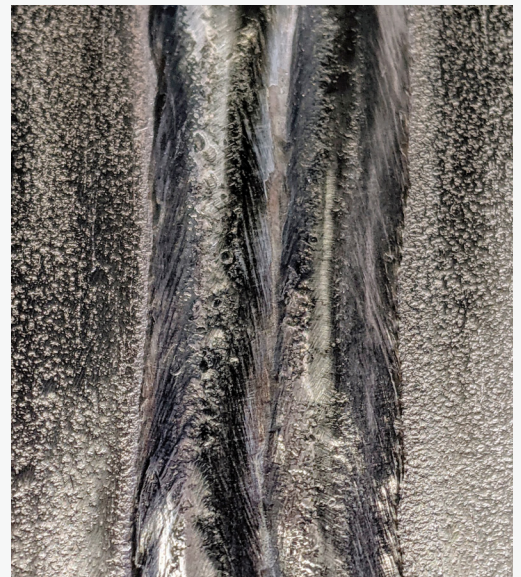
Spray pulse MIG welding close up.
